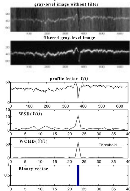
Fig. 5: Splits and cracks detection.
