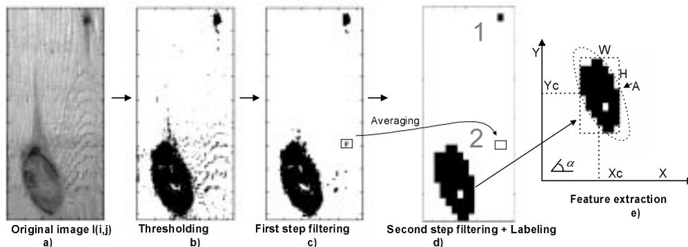
Fig. 3: Inspection of biological defects – algorithmic steps.
