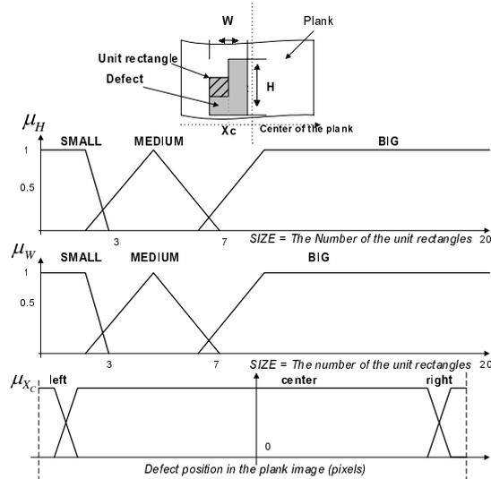
Fig. 6: Membership functions used for board defect description.
