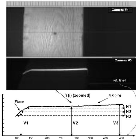
Fig. 4: Laser triangulation in function of wood board inspection and profile extraction.
